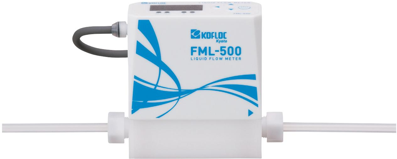
The FML-500 is a straight tube type ultrasonic flow meter for liquids. A new PFA material with excellent chemical resistance is used for parts in contact with the liquid, and the simple straight design facilitates maintenance without any obstacles inside the tube. It comes with a built-in display and the flow rate can be measured by connecting it to a power source. Flow rates up to a full scale of 5 L/min can be measured with high accuracy.
