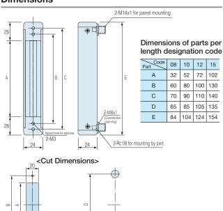
Mounting on the panel surface (Mount using accessory nuts)
